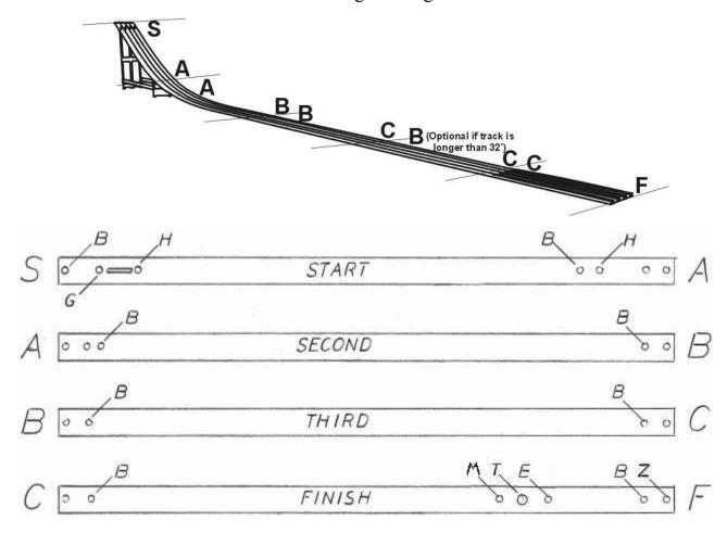
There are four different types of lane sections as indicated in the above drawing. Each section has its own unique hole pattern. Your first job with the 'Freedom' series is to nest together the sections to construct the specific width track you ordered. Begin by sorting the
